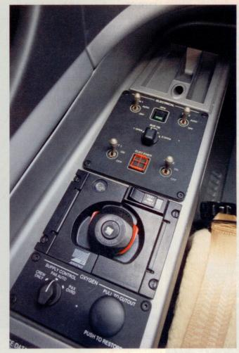
Embraer wanted the Phenom to be simple to operate, and the pilot's side panel proves it. Electrical and oxygen switches are kept to a minimum. Pushbutton switchlights are used for activating GPU and emergency electrical power sources.
