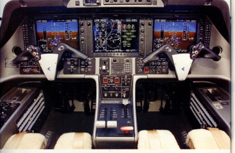
Embraer's signature ram's horn yokes and the Prodigy avionics suite dominate the Phenom 100 cockpit. The GFC 700 flight control system and integrated ESIS display are glareshield-mounted.
